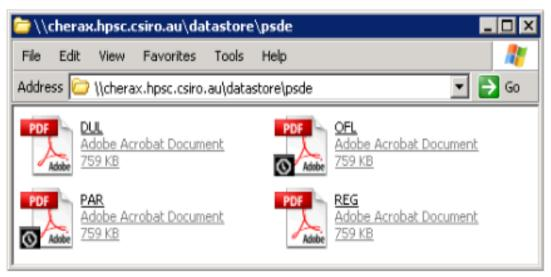
There's currently no good way for Windows users to do a bulk recall of offline files. They really need to run the dmget command on the DMF server or on a CXFS/NFS client of that server somehow.
