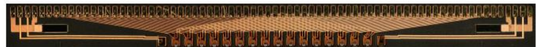
Figure 7: Plane View of LTO Chip Image Showing 16 Data Tracks, 2 Servo Readers and Connection Pads (at top) [5]
